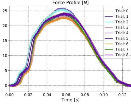
Fig. 7: Recorded data of nine impacts with the Panda. The end-effector soft-pad moves horizontally with 0.18 m/s, bumps orthogonally into a force sensor mounted to a wall, and pulls back upon contact detection.
