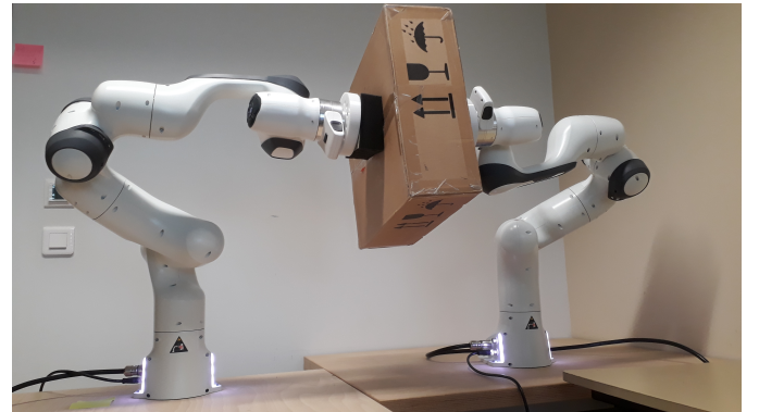
Fig. 2: Two Panda manipulators with soft, deformable pads attached to the end-effectors. We initiate contacts for swift box grabbing with pre-impact velocities of 0.61 m/s. The video is available at: https://youtu.be/dPLN87knF8
