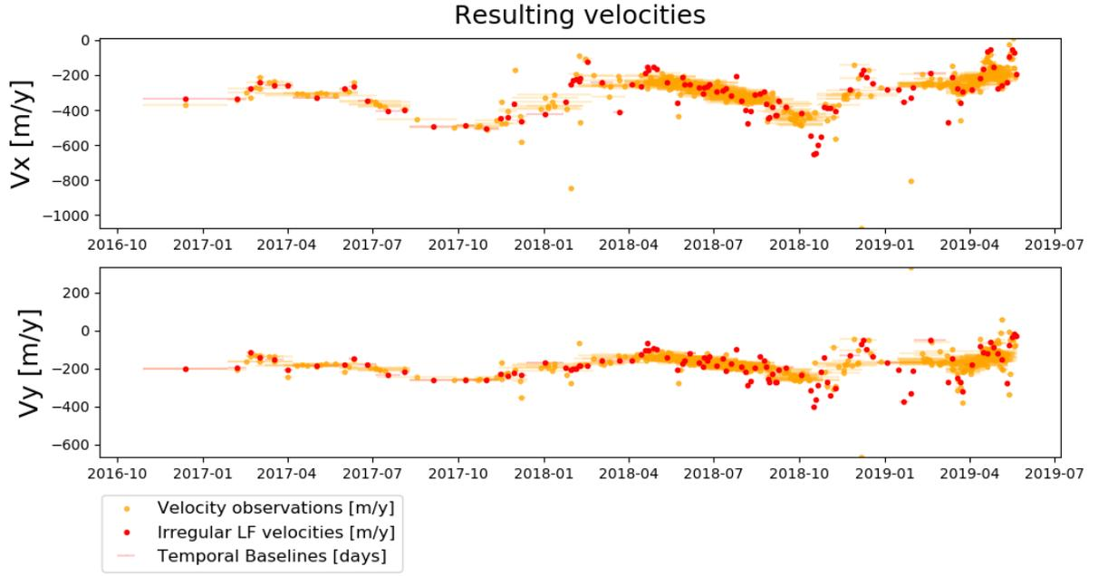
Figure 4. Velocity observations in gold overlaid with the Irregular Leap Frog time series obtained after temporal inversion in red for the point of coordinates  $(-43.532, 170.134)$  labeled as the blue point in Figure 1.
