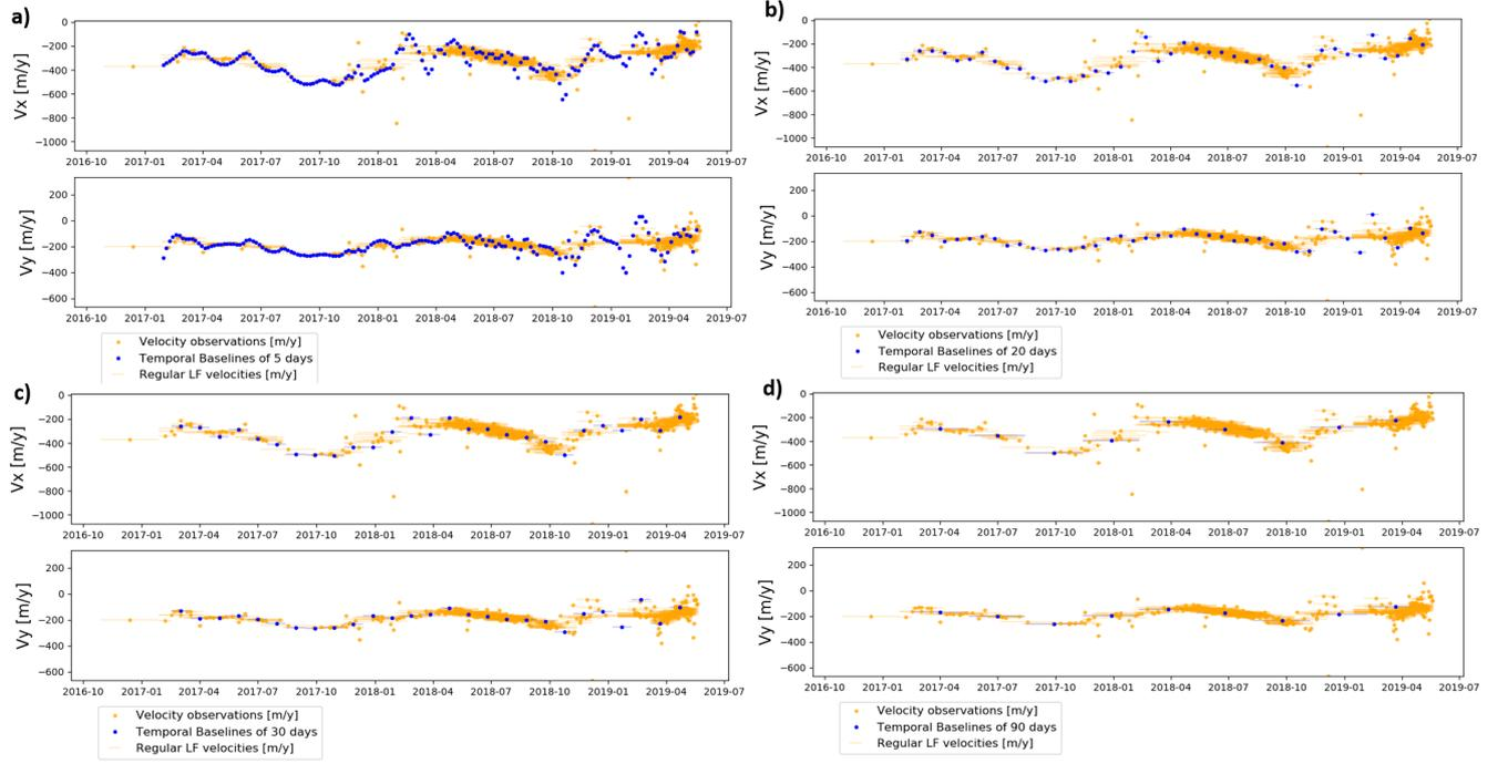
Figure 6. Velocity observations (in gold) overlaid with the RLF time series in blue for the point of coordinates  $(-43.532, 170.134)$  labeled as the blue point in Figure 1. The RLF time series have a temporal sampling of a) 5 days b) 20 days c) 30 days and d) 90 days.
