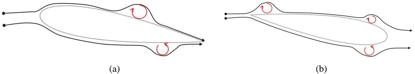
Fig.15 Sketch of the transition over two configurations. (a) Forward airfoil; (b) Reversed airfoil.
