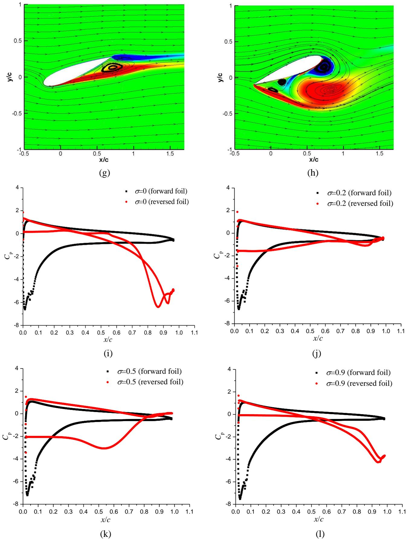
Fig.13 Flow structures and pressure distributions of forward and reversed airfoils. (a) and (b)  $\sigma=0$ ; (c) and (d)  $\sigma=0.2$ ; (e) and (f)  $\sigma=0.5$ ; (g) and (h)  $\sigma=0.9$ ; (i), (j), (k) and (l) Pressure coefficients.
