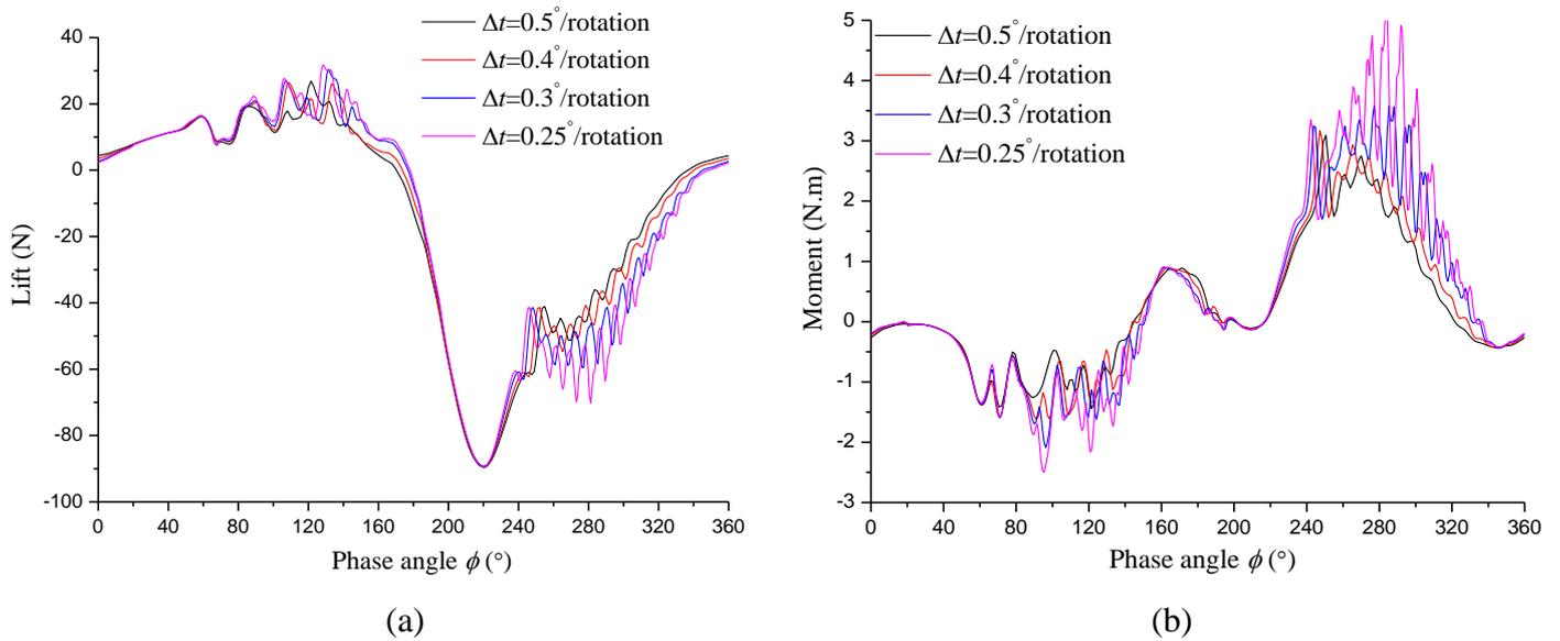
Fig.4 Plots of the instantaneous performance for different timesteps. The tested case is with the oscillating freestream of  $11.1 \cdot [1 + 0.5 \sin(\Phi - 135^\circ)]$  and reduced frequency of 0.036. (a) Lift; (b) Moment.
