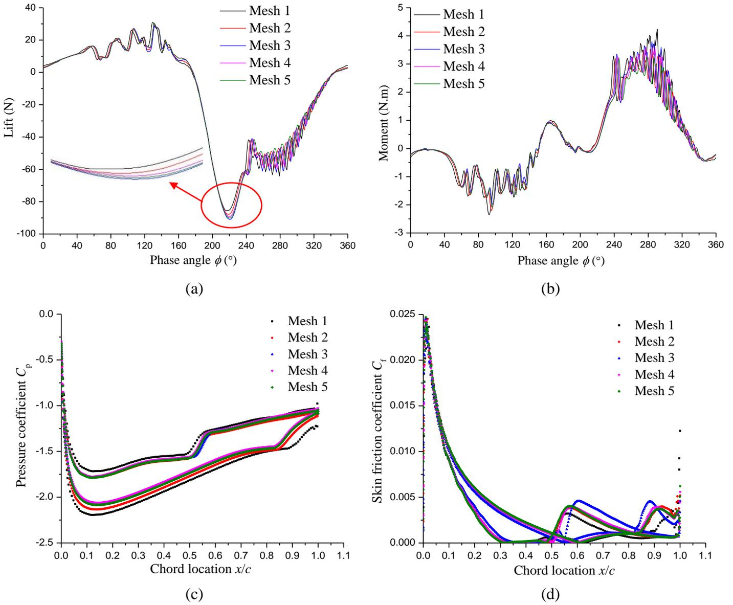
Fig.3 Plots of the instantaneous performance for different meshes. The tested case is with the oscillating freestream of  $11.1 \cdot [1 + 0.5 \sin(\Phi - 135^\circ)]$  and reduced frequency of 0.036. (a) Lift; (b) Moment; (c) Pressure coefficient; (d) Skin friction coefficient.
