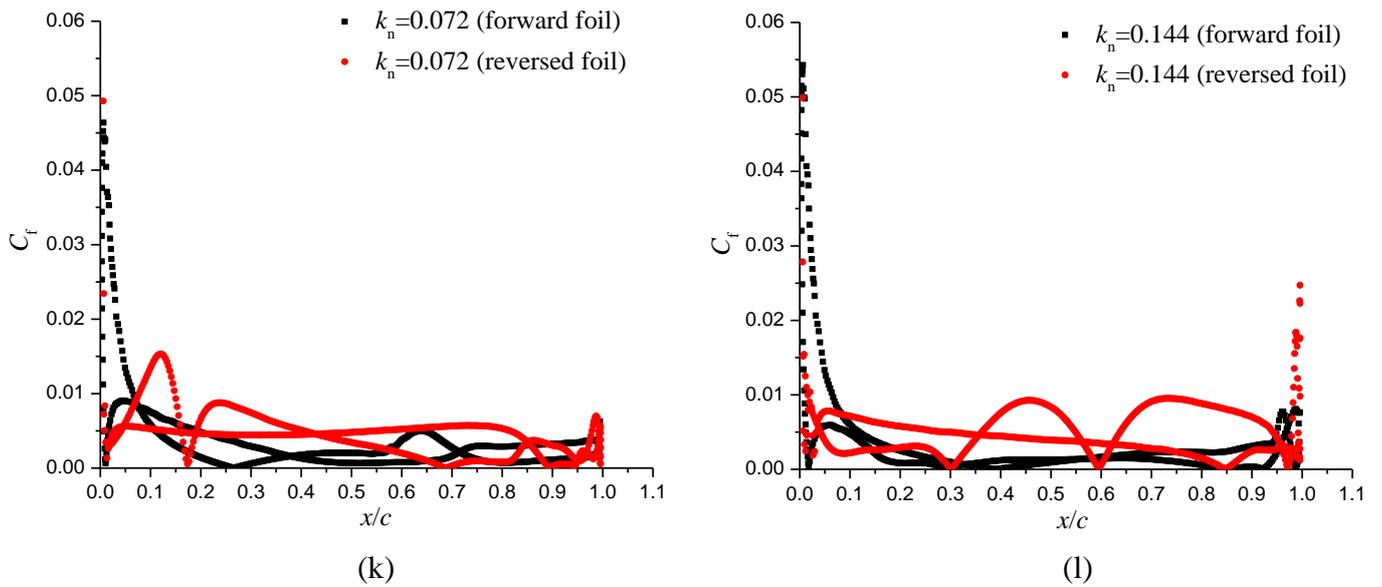
Fig.21 Transition and skin friction coefficients at  $\Phi=18^\circ$ . (a) and (b)  $k_n=0.020$ ; (c) and (d)  $k_n=0.036$ ; (e) and (f)  $k_n=0.072$ ; (g) and (h)  $k_n=0.144$ ; (i), (j), (k) and (l) Skin friction coefficients.
