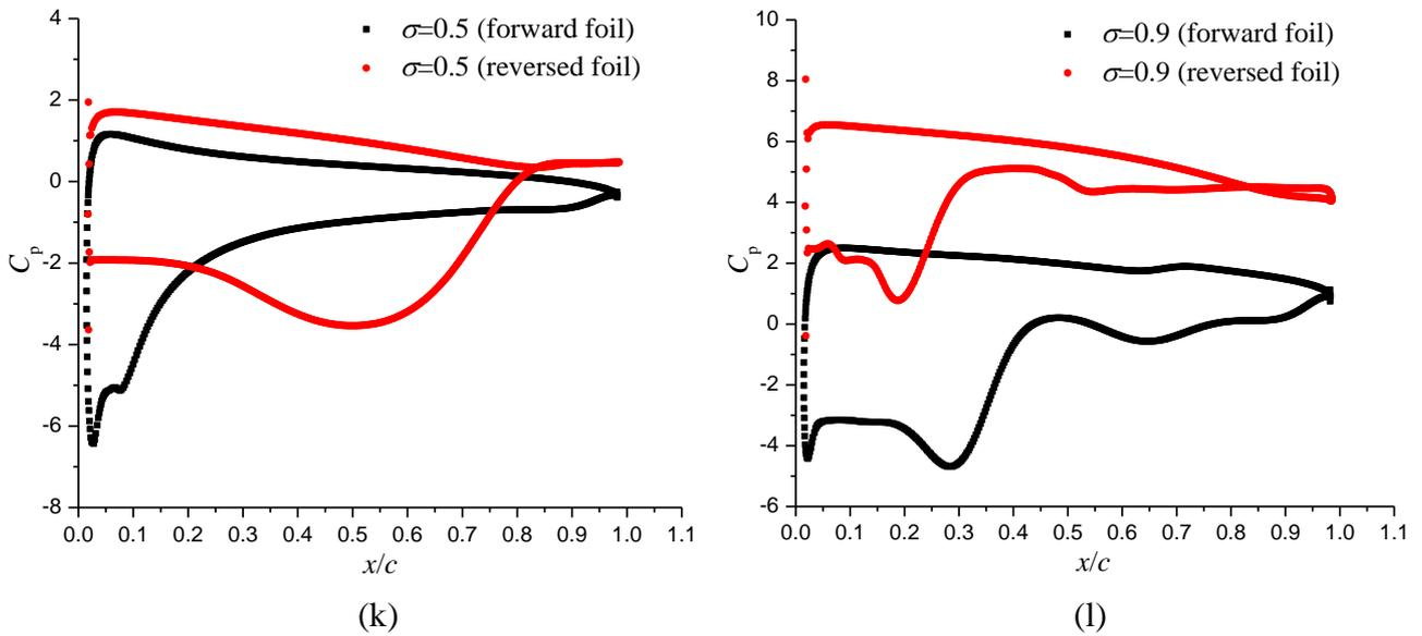
Fig.12 Flow structures and pressure distributions of forward and reversed airfoils. (a) and (b)  $\sigma=0$ ; (c) and (d)  $\sigma=0.2$ ; (e) and (f)  $\sigma=0.5$ ; (g) and (h)  $\sigma=0.9$ ; (i), (j), (k) and (l) Pressure coefficients.
