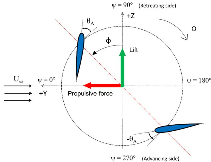
Figure.1 Sketch of cycloidal rotor system.
