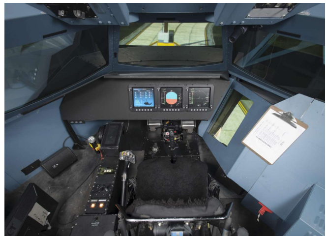
Figure 5. VMS R Cab cockpit emulating a utility class UH-60 sized helicopter.
