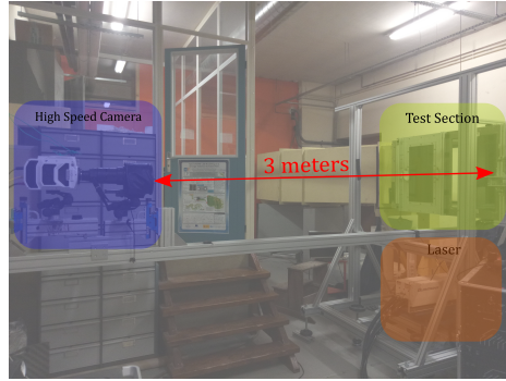
Fig. 3: PIV equipment. Configuration used to to image both upper and lower surfaces of the wing.
