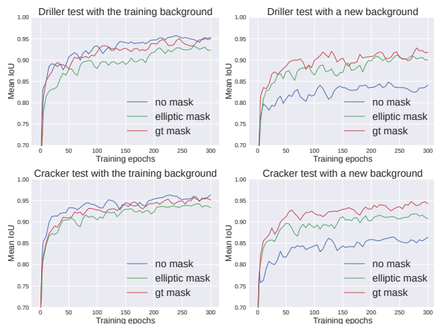
Fig. 18: Influence of the background: Comparison of the three masking strategies in terms of mean IoUs obtained during 300 training epochs for the driller and cracker objects. The left column shows the results obtained on test images with the same background as in the training images. The right columns show the results obtained on test images with an unseen background.
