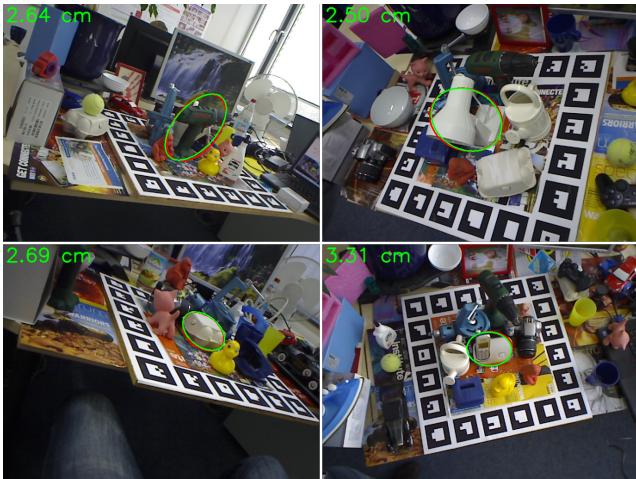
Fig. 11: Camera position estimation: Predicted ellipse (in green) for some objects of LINEMOD. The red ellipse (partially behind the green one) corresponds the ground truth projection of the ellipsoidal object model. The reported value in each image is the error of the estimated camera position.
