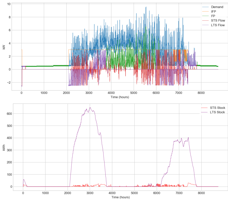
Figure 14: Solution of the RP-CF-SetUp model in case where the FP cost is 44.4 euros and the demand profile B is considered.
