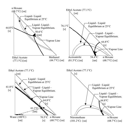
Figure 1. Residue curve maps of ternary systems n hexane – ethyl acetate – heterogeneous entrainer
