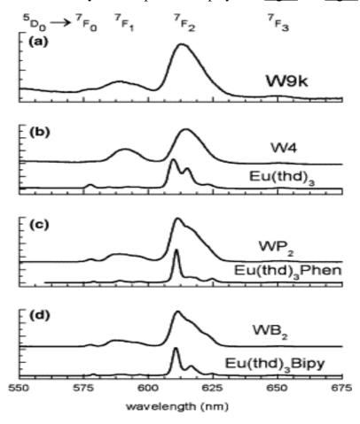
Fig. 5. Eu(III) emission spectra for (a) amorphous silica-europium oxide Eu@MCM-41 sample (W9k) and (b)–(d) upper curves, the grafted species W4, WP<sub>2</sub>, WB<sub>2</sub>; lower curves, the corresponding genuine complexes.
