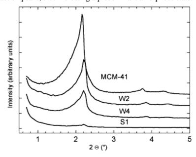
Fig. 2. X-ray diffraction patterns for pristine MCM-41 and variously loaded samples.
