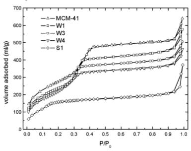
Fig. 1. Sorption isotherms of nitrogen at −196 °C.
