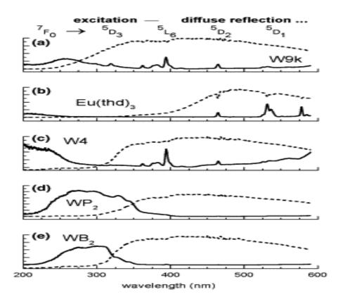
Fig. 6. Diffuse reflection spectra (dotted lines) and excitation spectra measuring the Eu(III) emission at 612 nm (solid lines) for (a) amorphous silica-europium oxide Eu@MCM-41 (W9k); (b) genuine Eu(thd)<sub>3</sub>; (c)–(e) the grafted species W4, WP<sub>2</sub>, WB<sub>2</sub>, respectively.
