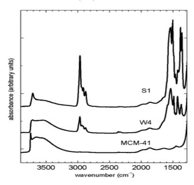
Fig. 4. IR absorption spectra recorded on self-supported wafers for unloaded MCM-41, and Eu(thd)<sub>x</sub>@MCM-41 hybrids (W4, S1) after degassing at 150 °C/ $10^{-2}$  Torr for 4 h.
