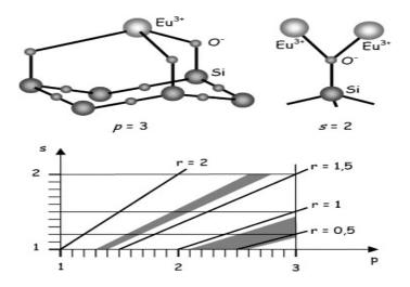
Fig. 7. Abacus showing the podality p versus the number s of Eu<sup>3+</sup> cations bond to the same SiO<sup>-</sup>, for different values of r = Eu/thd molar ratio. The grey zones correspond to the WI samples (right) and to CVI samples (left). The structural drawings illustrate a case of podality p = 3 about a tridymite fragment, and a case of s = 2 cations sharing the same SiO<sup>-</sup> group.
