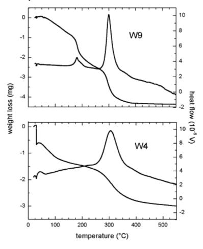
Fig. 3. TGA–DTA diagrams for wet impregnated  $Eu(thd)_x$ @MCM-41 hybrids, asprepared (W9), and degassed at 150 °C/10<sup>-3</sup> Torr for 12 h (W4).
