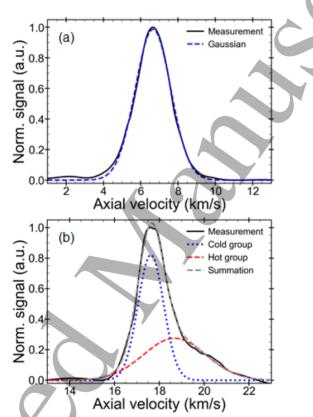
**Figure 6.** IVDFs fitted with Gaussian distribution at (a) z = -6 mm (single Gaussian), and (b) z = 60 mm (double Gaussian), respectively, at 300 V and 7.0 sccm. The blue dotted and red dashed curves in (b) represent the cold and hot ion groups, respectively. Their summation, denoted in gray, matches well with ( $R^2 > 0.995$ ) the measured IVDF, shown in black.
