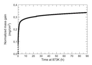
Fig. 1. Mass gain per unit area versus time during oxidation at 873 K of sample Cod2.
