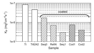
Fig. 2. Parabolic rate constants for the oxidation of pure Ti, of uncoated Ti6242, of a Al-Pt sequential coating processed from TIBA [2], and of the coated samples investigated in the present study.
