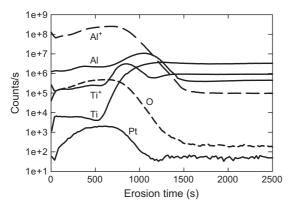
Fig. 4. SIMS element profiles as a function of erosion time for sample Cod2.
