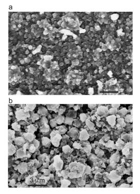
Fig. 3. SEM micrographs of the surface of the Cod2 sample, as deposited (a) and after oxidation (b).
