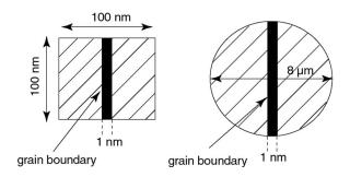
**Figure 10.** Sketches used for the modeling of the grain boundary diffusion of oxygen in nickel. (a) Grain boundary crossing a pixel in SIMS image mode, (b) grain boundary crossing the analyzed zone in SIMS concentration profile mode.
