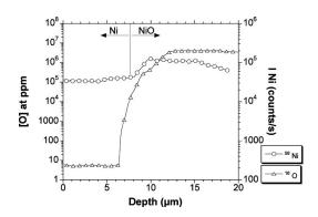
**Figure 4.** Reverse side SIMS profiles of  ${}^{16}O$  and  ${}^{54}Ni$  obtained in a 125- $\mu$ m-thick nickel foil–1 h/1000°C/laboratory air. Profiles obtained in a metallic grain.
