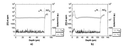
Figure 6. Reverse side SIMS profiles of  $^{16}$ O and  $^{58}$ Ni obtained in a 1-mm-thick nickel foil-48 h/1000°C/ laboratory air. (a) Profiles obtained in a metallic grain, (b) profiles obtained in a metallic grain boundary.
