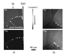
**Figure 7.** SIMS images of <sup>16</sup>O and <sup>58</sup>Ni obtained in 1-mm thick nickel foils oxidized 48 h at 1000°C in laboratory air cross sections. (a) Metal/oxide scale interface, (b) 500  $\mu$ m under the metal/oxide scale interface. Note that, in each case, nickel grain boundaries have been marked by dashed lines.
