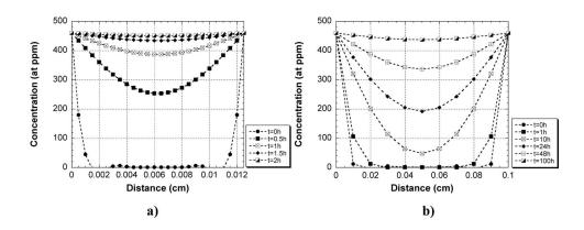
Figure 3. Calculations of the oxygen diffusivity in solid nickel at 1000°C as a function of time. (a) 125-µm-thick foil, (b) 1-mm-thick foil. The diffusion coefficient D ( $D = 9.13 \times 10^{-9}$  cm<sup>2</sup> s<sup>-1</sup>) and the solubility  $C_s$  ( $C_s = 460$  at ppm) obtained by Park and Alstetter<sup>10</sup> at 1000°C were used for the calculations.
