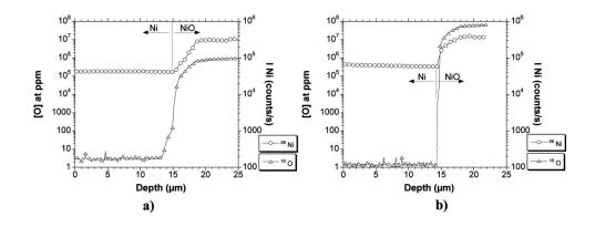
Figure 5. Reverse side SIMS profiles of  $^{16}$ O and  $^{58}$ Ni obtained in a 125- $\mu$ m-thick nickel foil—100 h/ 1000°C/laboratory air. (a) Profiles obtained in a metallic grain, (b) profiles obtained in a metallic grain boundary.
