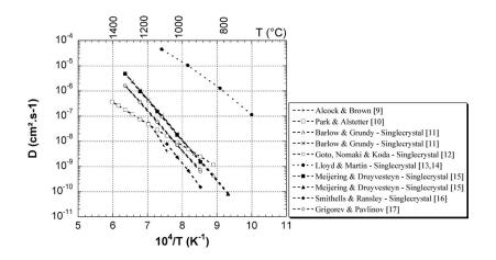
**Figure 2.** Diffusivity of oxygen in solid nickel at high temperature (literature data).
