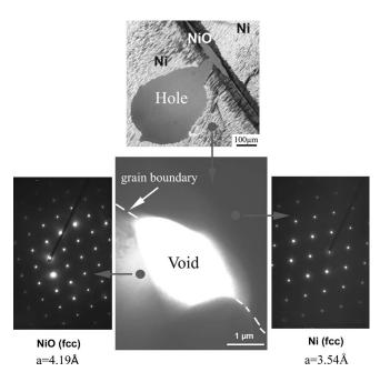
**Figure 8.** Presence of nickel oxide particles in a metallic grain boundary 200  $\mu$ m under the metal/oxide scale interface. Nickel foil B oxidized 48 h at 1000°C in air (TEM investigation).
