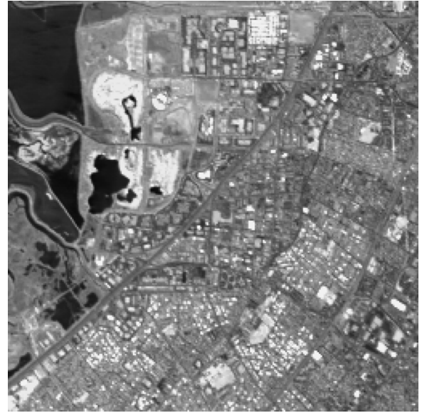
Fig. 5. Moffett3 with uneven zones. Color composition (shown in grayscale) of bands 90 (1211.33 nm), 40 (731.21 nm), and 20 (557.07 nm). This area contains man-made targets and vegetation.
