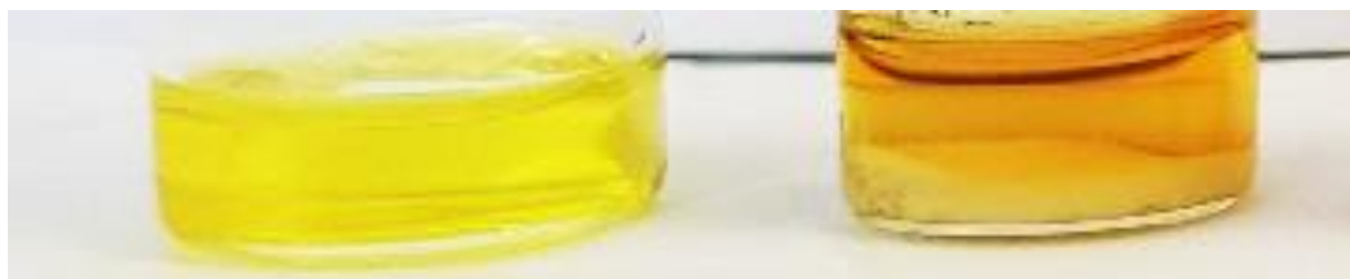
Figure S2 Photography of the solutions before (left) and after (right) 14 days driving to the single-crystal growth of \text{Cs}_2\text{PbCl}_2\text{I}_2 -type materials.
