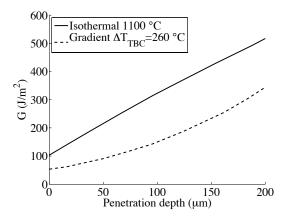
Figure 1.29: Energy release rate (G) as a function of CMAS infiltration depth for a delamination crack at the base of a YSZ TBC ( $T_{surface} = 1300 \text{ °C}$ ,  $T_{bond \ coat} = 1040 \text{ °C}$  and  $T_{backside} = 800 \text{ °C}$ ); comparison with a TBC isothermally heated at 1100 °C (based on information from reference [140])
