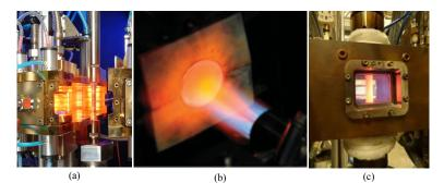
Figure 1.24: TMF testing of TBC in presence of gradient (a) TGMF [13], (b) Burner rig [103] and (c) Combustion environmement in TGMF condition [106]
