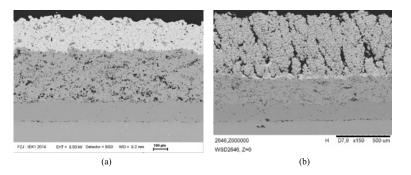
Figure 1.8: SEM micrographs of (a) an APS  $Gd_2Zr_2O_7/YSZ$  and (b) a SPS  $La(Al_{0.25}Mg_{0.5}Ta_{0.25})O_3/YSZ$  double layer system.
