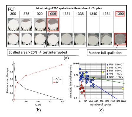
Figure 1.22: Effect of thermal furnace cycling for EB-PVD, (Ni,Pt)Al bondcoat and first generation single crystal superalloy. (a) Appearance of TBC spallation observed on button shape specimens as a function of cycle number, [60], (b) evolution of critical strain,  $\varepsilon_c$ , at spallation and associated damage, D, as a function of the time spent at high temperature (adapted from [40]), and (c) interfacial toughness as a function of the number of furnace cycles and temperature [195]
