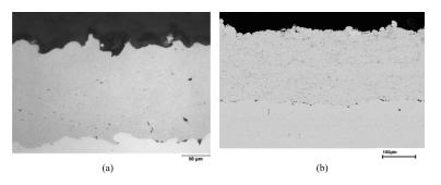
Figure 1.4: SEM micrograph of a VPS (a) and a HVOF bond coat (b).
