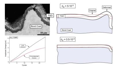
Figure 1.34: Rumpling modeling by initial defect meshing and strain increase associated to oxide growth in plane and out of plane (thickening and lengthening strain) and thermal gradient mechanical fatigue (TGMF) loading [161]
