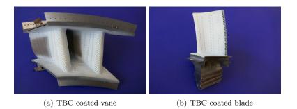
Figure 1.1: TBC coated vane (a) and blade (b) of a GP7000 aero engine
