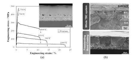
Figure 1.12: Tensile test on free standing BC specimens for (Ni,Pt)Al coating, (a) stress-strain curves at different temperatures and (b) fracture surfaces of specimens comprising SX substrate material, BC, and inter diffusion zone between SX and BC (right top) and BC only specimen (right bottom) [182]
