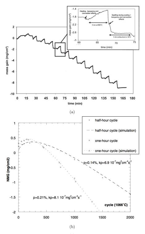
Figure 1.30: Net mass gain evolution (a) measured experimentally in situ to derive the oxide growth kinetic  $k_p$  and probability of oxide spallation p [121] and (b) measured experimentally ex situ by weighting of specimen after each cycle and modeled by  $p - k_p$  [142]
