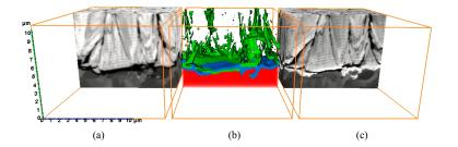
Figure 1.19: Reconstructed volume from FIB-SEM serial sectioning (Box size: 11  $\mu$ m x 14.2  $\mu$ m x 18.88  $\mu$ m). Segmentation of the different phases BC, TGO, TC, and cracks or voids was performed by using images from Backscatter Electron (a) and Secondary Electron (c) detectors. In (b), the BC is displayed in red, the TGO in blue, cracks, respective voids in green, and the TC transparent to allow for viewing the structure of inter-columnar gaps (courtesy of A. Dennstedt).
