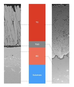
Figure 1.2: Typical TBC systems comprising ceramic TC, TGO, and metallic BC applied on a superalloy substrate. Left: EB-PVD processed TC with a (Ni, Pt)Al BC (courtesy of Lara Mahfouz) Right: APS processed TC with a MCrAlY BC adapted from [130]
