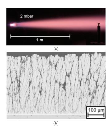
Figure 1.7: (a) Photo of the plasma plume in the PS-PVD process, (b) SEM micrograph of the columnar structure of PS-PVD YSZ coating (courtesy H. Moitoux, S. Rezanka, Forschungszentrum Jülich).
