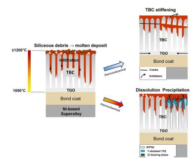
Figure 1.25: CMAS- induced degradation mechanisms of EB-PVD thermal barrier coatings
