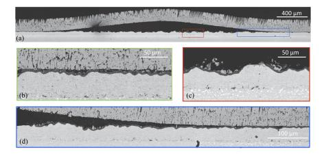
Figure 1.21: Interfacial defect introduced by LASAT in the as-processed condition and observed after 2000 thermal cycles at 1100 °C, (a) global view of the blister, (b) detail view out of (a): interface evolution without interaction with the initial defect, (c) detail view, see red rectangle in (a): initial area of decohesion, (d) detail view, see blue rectangle in (a): evolution in the vicinity of the interfacial crack tip (courtesy of Lara Mahfouz)
