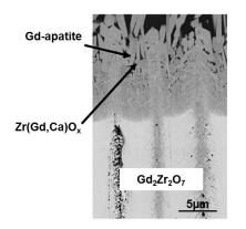
Figure 1.26: SEM micrograph showing the sealing of the intercolumnar gaps of an EB-PVD  $Gd_2Zr_2O_7$  coating by the combination of Gd-apatite and Zr(Gd,Ca)Ox crystalline phases (based on information from [101])
