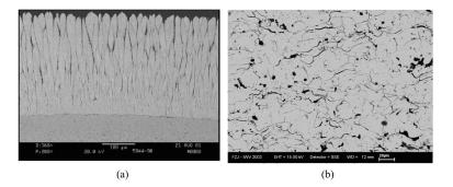
Figure 1.5: SEM micrographs of EB-PVD [64] (a) and APS (b) coatings.
