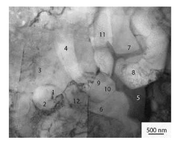
Figure 6. Bright field image of the precipitate in the grain boundary of sample 2. The numbers refer to locations of EDX measurements.
