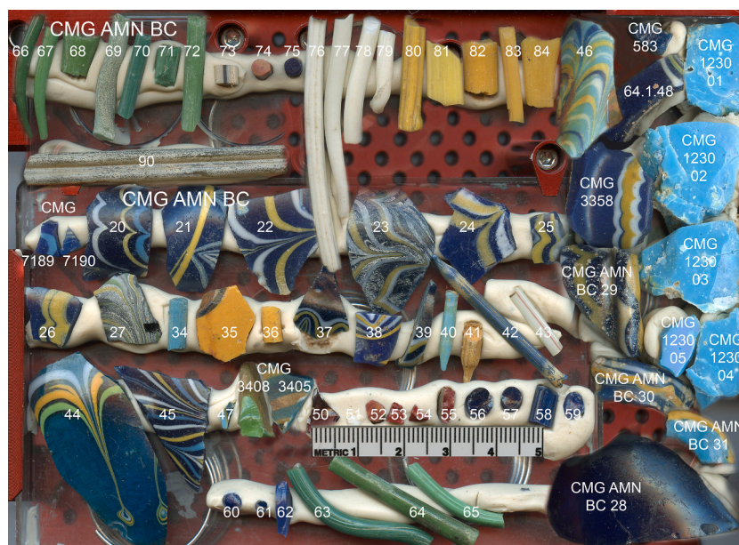
Fig. 2. Representative Late Bronze Age vessel fragments and production debris mounted in the LA-ICP-MS sampling cell. Most of these samples are from Amarna, along with copper-blue ingot fragments from Tell Brak. For sample identification see Table S2.
