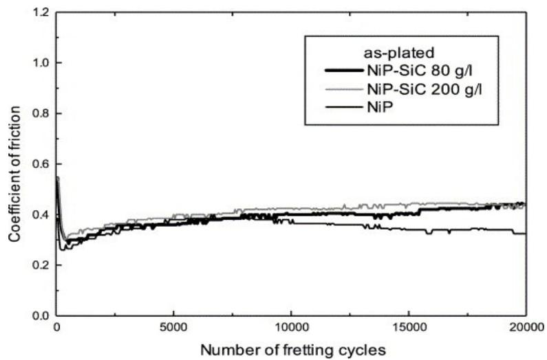
Fig. 12. Coefficient of friction after fretting on heat-treated NiP and NiP–SiC coatings (500  $\mu\text{m}$ , 2 Hz, 10 N, 20 000 cycles).
