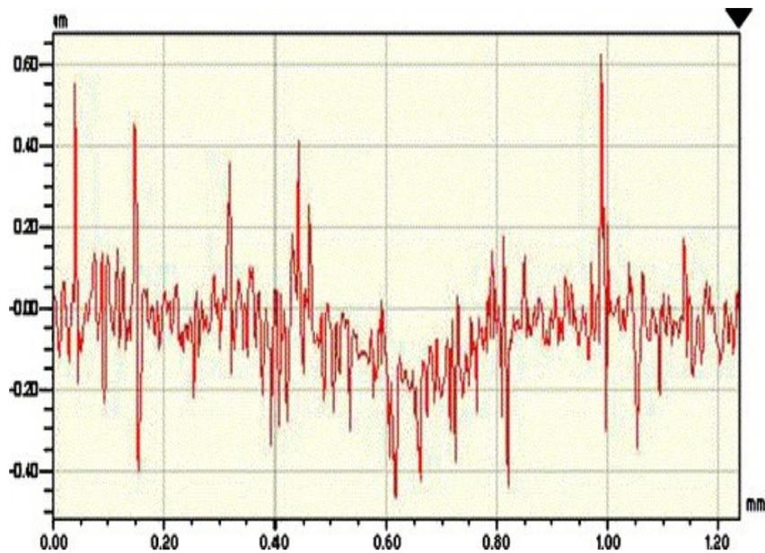
Fig. 17. X-profile of the wear track of heat-treated NiP–SiC, 200 g/l at the bi-directional sliding test (40 000 fretting contacts, 10 N, 2 Hz, ambient air 50% RH and 23 °C).
