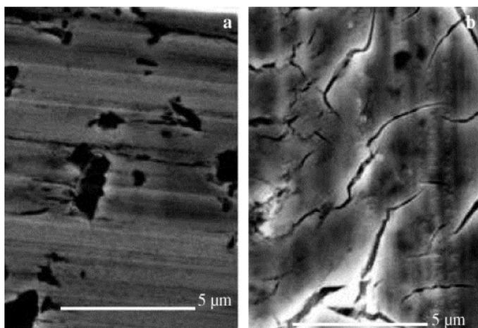
Fig. 6. Detail of Fig. 3 microcracks in the wear track near the rim.
