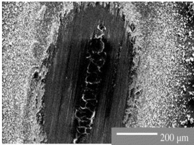
Fig. 2. Back scattered image and elemental mapping of the wear track in as-plated NiP–SiC coating, 600 nm 80 g/l: (a) backscattered image at the centre of wear track after fretting: 10 N, 2 Hz, 500  $\mu$ m, 20 000 cycles; (b) elemental mapping of aluminum; (c) elemental mapping of oxygen.
