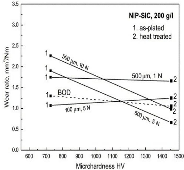
Fig. 15. Wear rate after uni- and bi-directional (40 000 fretting contacts, ambient air 50% RH and 23 °C) sliding tests vs. Vickers hardness for as-plated and heat treated pure NiP coatings. Dotted line correspond to data for uni-directional sliding test (15 000 contacts, 2 N, 0.15 m/s, 1 Hz, ambient air 50% RH and 23 °C).
