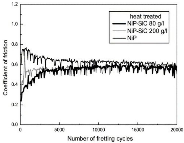
Fig. 11. Coefficient of friction after fretting on as-plated NiP and composite NiP–SiC coatings (500  $\mu\text{m}$ , 2 Hz, 10 N, 20 000 cycles).
