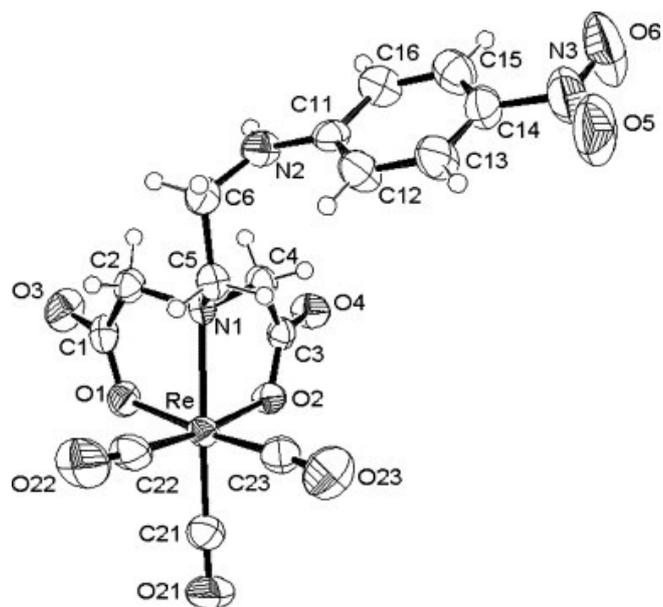
Fig. 2. ORTEP drawing of the  $[\text{Re}(\text{CO})_3(\text{L}^3)]^-$  complex anion (**3**) with numbering scheme. Thermal ellipsoids are drawn at the 30% probability level.
