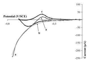
Fig. 6. Theoretical fitting of cyclic voltammogram 0.2 V/s for PEG/PEI/P450<sub>BM3</sub>/PEI electrodes: (a) experimental current; (b) theoretical residual current; (c) current due to P450<sub>BM3</sub> electrochemistry only.
