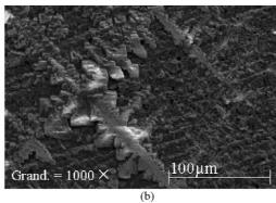
Fig. 3. SEM views of coated PG electrodes, magnification of  $\times 1000$ : (a) {PG/PEI/P450<sub>BM3</sub>/PEI} layer-by-layer film and (b) PG/PEI/P450<sub>BM3</sub>/PEI "cast polyion" film.
