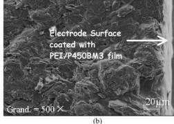
Fig. 2. SEM cross-section views of coated PG electrodes, magnification of  $\times 500$ : (a)  $\{PG/PEI/P450_{BM_3}\}$  layer-by-layer film and (b)  $PG/PEI/P450_{BM_3}$  "cast polyion" film.
