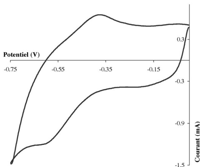
Fig. 9. Cyclic voltammogram at 0.2 V/s for a felt RVG/PEI/P450<sub>BM3</sub>/PEI electrode in Tris-HCl pH 7.5.
