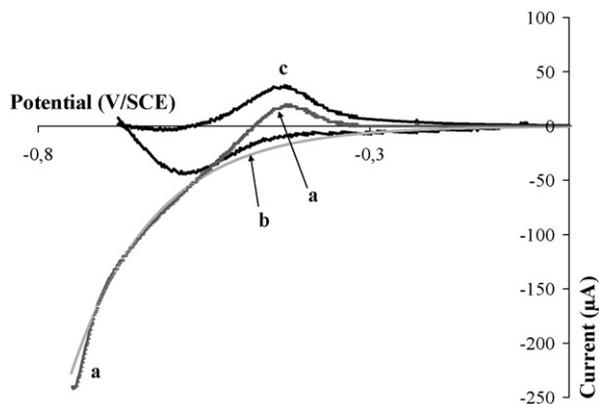
Fig. 6. Theoretical fitting of cyclic voltammogram 0.2 V/s for PEG/PEI/P450<sub>BM<sub>3</sub></sub>/PEI electrodes: (a) experimental current; (b) theoretical residual current; (c) current due to P450<sub>BM<sub>3</sub></sub> electrochemistry only.
