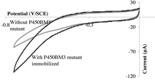
Fig. 4. Cyclic voltammograms at 0.01 V/s for PG/PEI/P450<sub>BM<sub>3</sub></sub>/PEI and PG/PEI electrodes; 15 mL air in 20 mL buffer pH 7.5.
