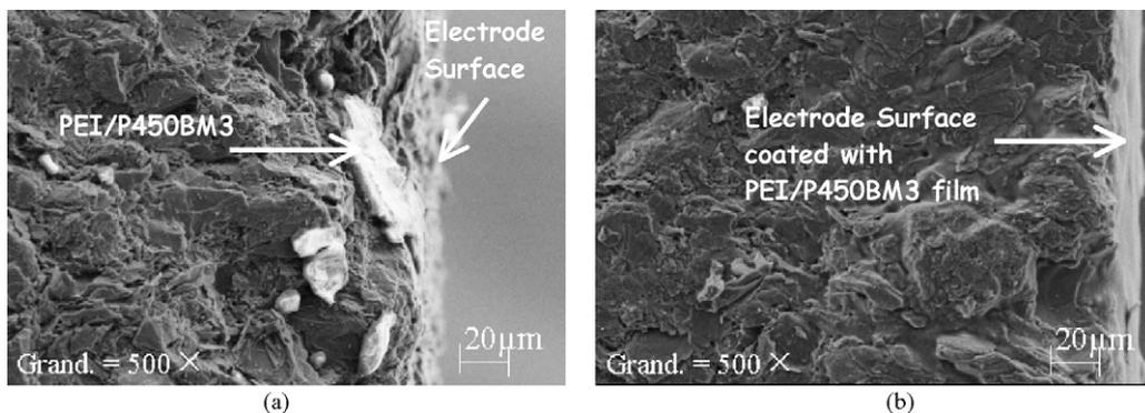
Fig. 2. SEM cross-section views of coated PG electrodes, magnification of  $\times 500$ : (a) {PG/PEI/P450<sub>BM3</sub>} layer-by-layer film and (b) PG/PEI/P450<sub>BM3</sub> “cast polyion” film.
