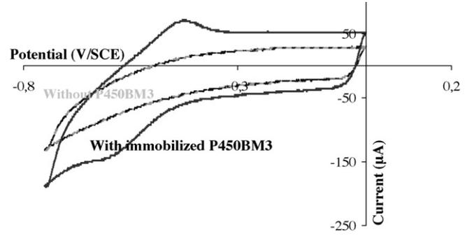
Fig. 5. Cyclic voltammograms on PG electrodes at 0.2 V/s in the absence of oxygen in pH 7.5 buffer with PG/PEI/P450<sub>BM<sub>3</sub></sub>/PEI and PG/PEI selectrodes.
