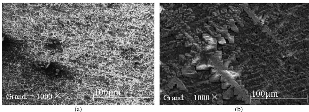
Fig. 3. SEM views of coated PG electrodes, magnification of  $\times 1000$ : (a) {PG/PEI/P450<sub>BM3</sub>/PEI} layer-by-layer film and (b) PG/PEI/P450<sub>BM3</sub>/PEI “cast polyion” film.
