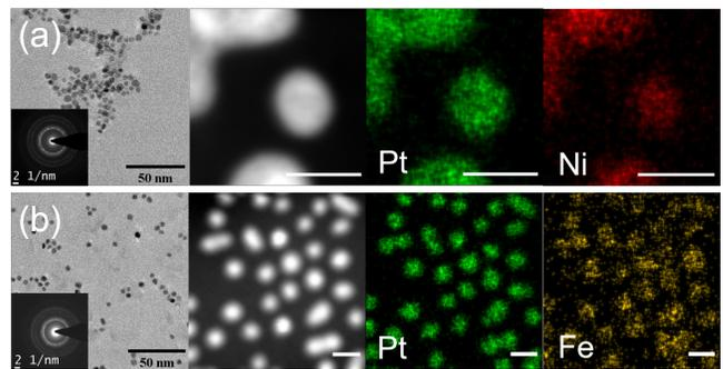
FIG. 3. (a) NiPt (Ni=(56 $\pm$ 6) %at, Pt= (44 $\pm$ 6) %at.) and (b) FePt (Fe=47 $\pm$ 7 %at., Pt= 53 $\pm$ 7 %at.) bimetallic NPs. (Left) Bright-field micrograph of sample representative of the NP dispersion for all samples studied. As inset, electron diffraction patterns corresponding to FCC structure. (Center) HAADF-STEM image of NPs. (Right) EDX chemical mappings showing the spatial correlation between the different elements present in a set of NPs of the sample. (Scale bar = 5 nm)
