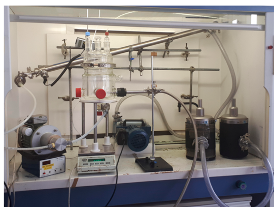
Figure 2. Lab-scale installation to determine the feasibility of DCM purification by pervaporation.
