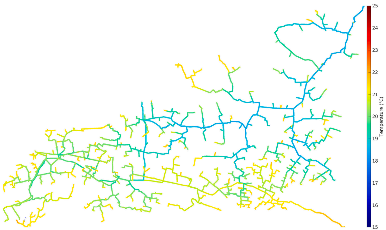
Fig. 12. Modeled water temperature in the raw water network (presented in 2) on the 30th of June 2018 at midday (soil temperature is .21.6°C).
