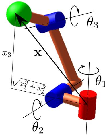
Figure 2: An example of orthogonal 3R serial robot
