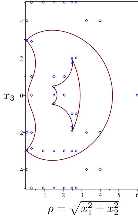
Figure 3: Projection on the plane  $(\rho, x_3)$  of the set atypical values (red curve) of an orthogonal 3R serial robot and the points (blue diamonds) of the sample set  $\mathcal{P}$  that meets every connected component of the complementary of  $\overline{\text{atyp}(\mathcal{R})}^z$ .
