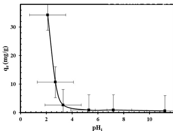
**Fig. 4.** Effect of pH on the PS biosorption onto FS ( $[PS]_0 = 35 \text{ mg L}^{-1}$ ,  $m(\text{FS}) = 250 \text{ mg}$ ,  $V = 200 \text{ mL}$ , contact time = 60 min,  $T = 296 \text{ K}$ )
