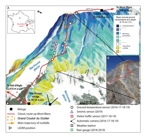
**Figure 1.** Study site and multi-method monitoring system at the Grand Couloir du Goûter. (a) Permafrost map from the modelling of Magnin et al. (2015) (aerial photography © Microsoft) showing the locations of the classic route up Mont Blanc on the west face of the Aiguille du Goûter (in red) and the instruments set up in the area. The years in which the sensors were present are indicated. (b) Picture of the couloir taken by the automatic camera (4 August 2019).
