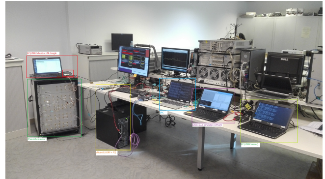
FIGURE 4. The Emuradio4Rail platform with one LTE bearer emulated by OAI and FPGA based channel emulator in the IKERLAN laboratory
