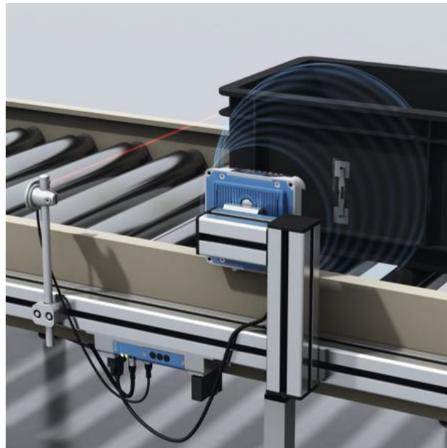
Figure 2: Application of the RFID system in material handling system.
