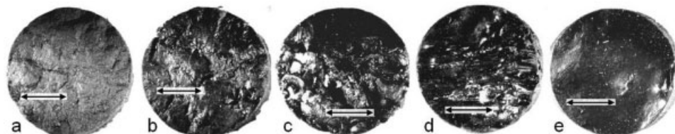
FIG. 1. Film morphology according to extruder die temperature (a: 85°C, b: 105°C, c: 125°C, d:145°C, and e: 160°C). Scale arrow length: 5 mm.
