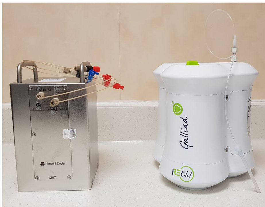
FIGURE 1 | Radiopharmaceutical grade germanium-68 ( ^{68}\text{Ge} )/gallium-68 ( ^{68}\text{Ga} ) generators from left to right: GalliaPharm ® , Galli Ad ® , and GeGant ® .
