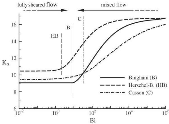
Fig. 8. Metzner–Otto parameter  $K_s$  for viscoplastic fluids in Taylor–Couette flow. Vertical lines: transition Bingham number  $Bi^*$  for the three models studied (case  $s=0.5$  for Bingham, Casson and Hershel Bulkley with  $n=0.5$ ).
