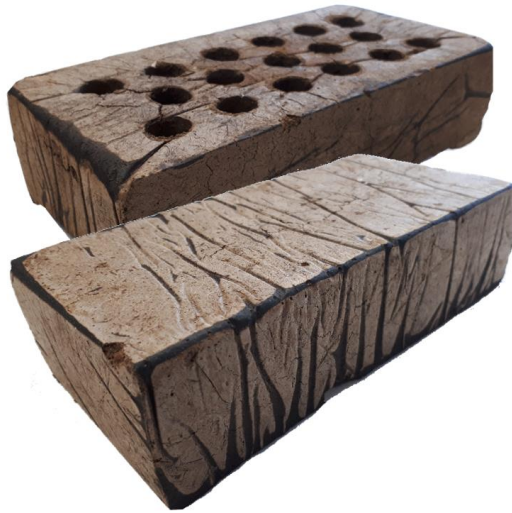
Figure 6. Examples of full and hollowed SSCC-40 bricks ( 220 \times 100 \times 60 \text{ mm}^3 ).
