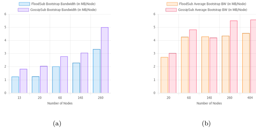
Figure 5. DSDCA: Floodsub vs Gossipsub Bootstrap Bandwidth, (a) 3 Swarms DSDCA in Mb/node, (b) 4 Swarms DSDCA in Mb/node
