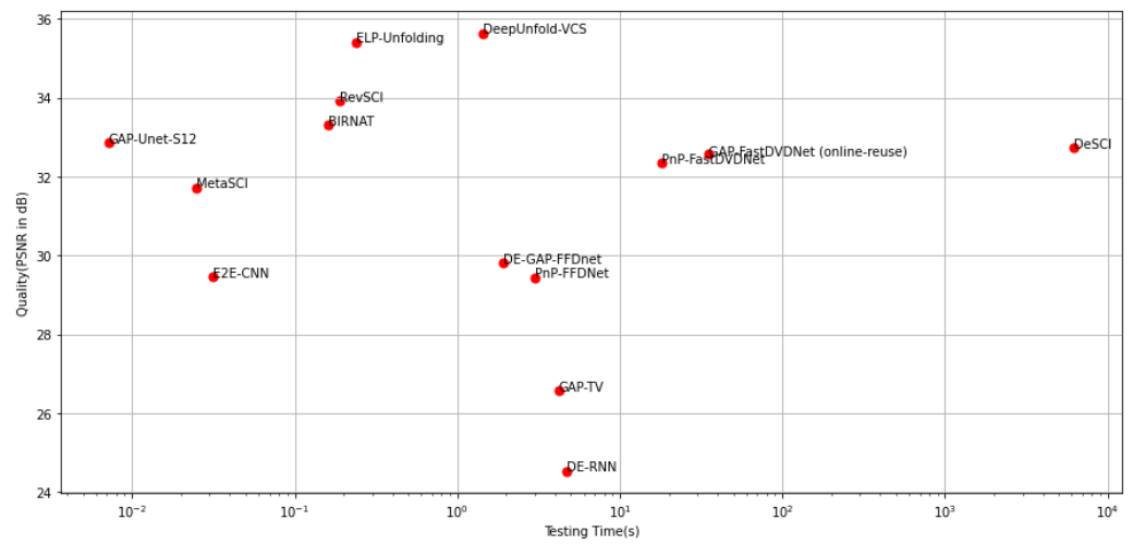
Figure 13. Trade-off between quality (in PSNR) and testing time of several VCS reconstruction algorithms.
