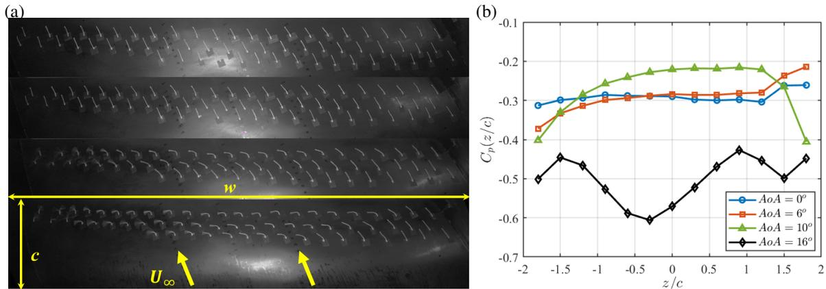
**Fig. 3** (a) Tuft visualisation for  $AoA = [0, 6, 10, 16]^\circ$  increasing from top to bottom view. (b) Pressure coefficient distribution along the span at  $x/c = 70\%$ . Both figures are shown for  $AoA = [0, 6, 10, 16]^\circ$  and  $Re_c \approx 10^6$ .
