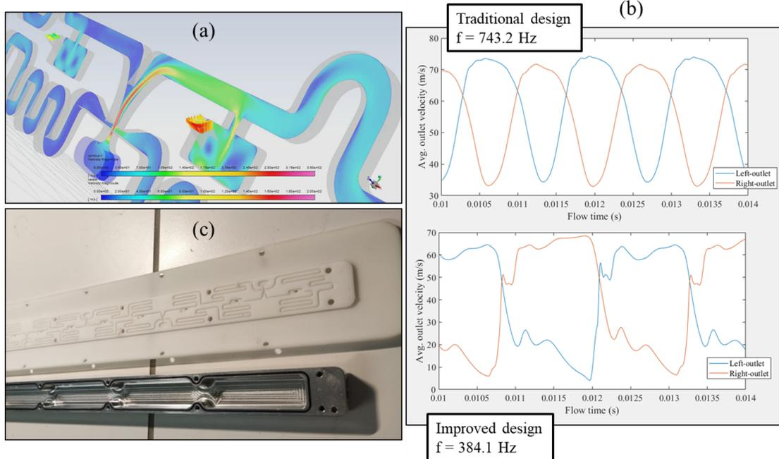
**Fig. 6** (a) Velocity field in the mid plane and velocity vectors at the outlet of a PJA assembly, (b) average velocity profile at the outlets of traditional (top) and improved PJA (bottom) designs with feedback loop length of 190 mm and 137 mm respectively and (c) 3D printed sample of a PJA assembly.
