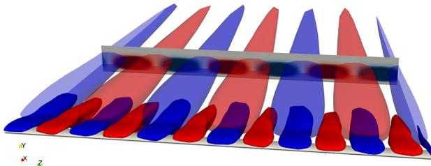
**Fig. 9** Growth rate sensitivity  $\nabla_F \lambda$  of the stall mode in the streamwise directions for  $\alpha = 20^\circ$  and  $Re = 400$ . The red (respectively, blue) isocontours represents positive (respectively, negative) values corresponding to one tenth of the maximal absolute value. The opaque isocontours illustrate the real part of the streamwise velocity for the corresponding direct stall mode, while the upstream slice depicts the associated streamwise vorticity.
