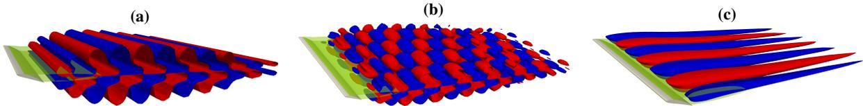
**Fig. 5** Real part of the streamwise velocity for (a) the two-dimensional VK mode ( $\beta = 0$ ), (b) the three-dimensional VK mode ( $\beta = \pi/2$ ) and (c) the ST mode ( $\beta = 3\pi/4$ ). The red (respectively, blue) isocontours represents positive (respectively, negative) values corresponding to one tenth of the maximal absolute value, while the opaque green isocontour represents the locus of the points where the streamwise velocity of the base flow is zero, i.e.  $U = 0$ .
