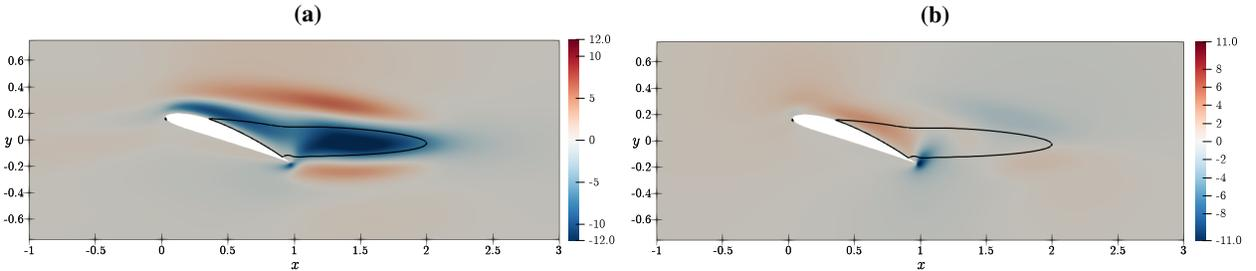
**Fig. 7** Growth rate sensitivity  $\nabla_F \lambda$  of the 2D VK mode in (a) the streamwise and (b) cross-stream directions for  $\alpha = 20^\circ$  and  $Re = 200$ . The black solid line corresponds to the isocontour  $U = 0$ .
