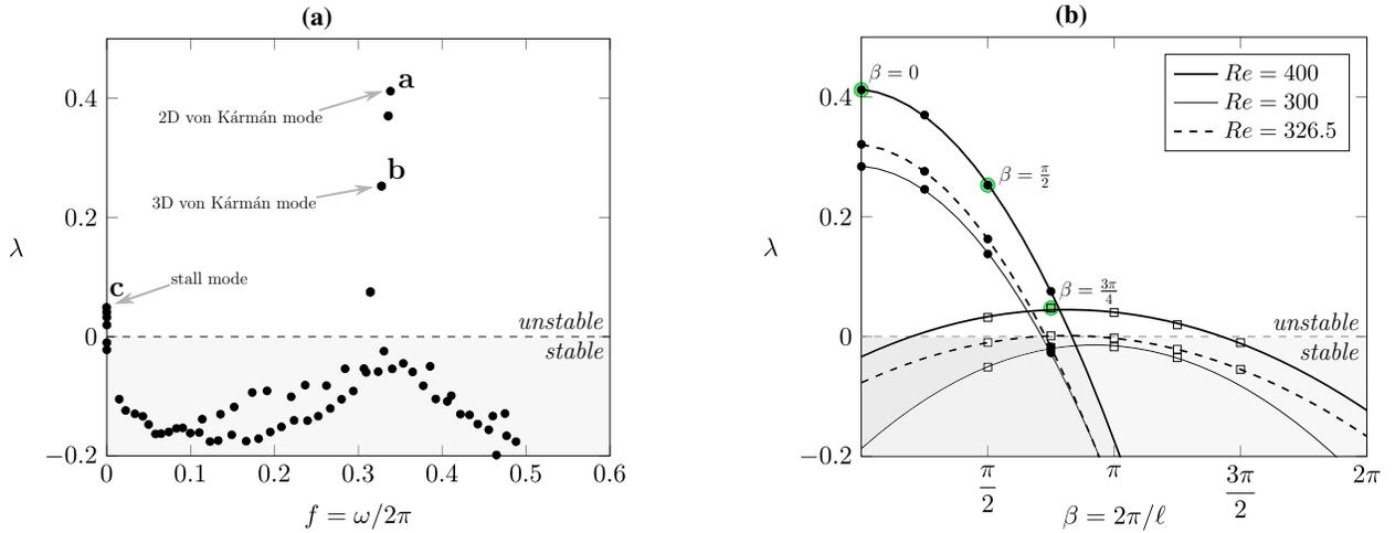
**Fig. 4** (a) Spectrum relative to the base state of Fig. 3 for  $\alpha = 20^\circ$  and  $Re = 400$  and (b) the growth rate as a function of the spanwise wavenumber. The bold letters in Fig. (a) and the green dots in Fig. (b) indicate the corresponding direct eigenmodes illustrated in Fig. 5.
