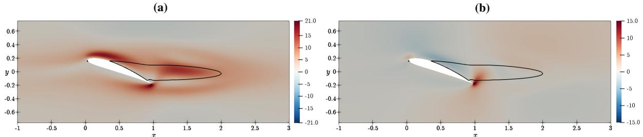
**Fig. 8** Frequency sensitivity  $\nabla_F \lambda$  of the 2D VK mode in (a) the streamwise and (b) cross-stream directions for  $\alpha = 20^\circ$  and  $Re = 200$ . The black solid line corresponds to the isocontour  $U = 0$ .
