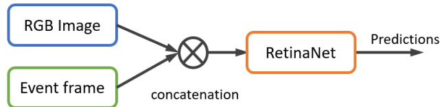
Fig. 4. Early Fusion: In this network the RGB and the event-voxels are concatenated before being fed to the RetinaNet.
