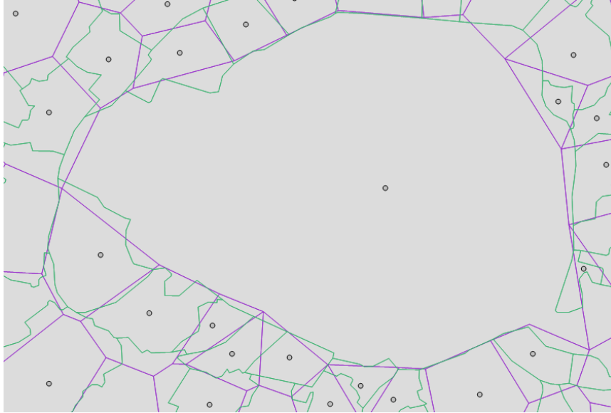
Figure 2-31: Manual adjustment in the Voronoi layer for large central municipalities surrounded by “small” peripheral municipalities
