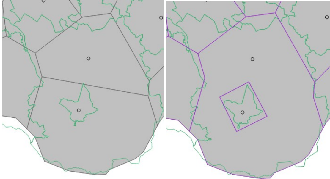
Figure 2-29: Manual adjustments in the Voronoi layer for urban object surrounded by rural territories
