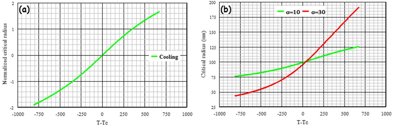
FIG. 3. Evolution of the critical crystal size for the  $t \rightarrow m$  SPT during the cooling process. (a) The normalized critical radius is plotted according to Eq. (12) taking into account the value of  $\lambda$  and the critical temperature that have been determined experimentally for cooling (Table I). (b) Critical radius considering a hypothetical value of the mean crystal size (100 nm) and standard deviations of the size distribution of 10 and 30 nm.
