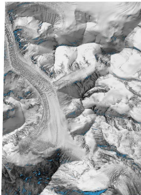
Figure A2. Subset of the SRE product on which the TopCos no data mask is applied. Blue pixels signify no data due to the \cos(\gamma) threshold. VEN \mu S image of 27 March 2018.
