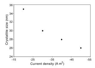
Fig. 9. Effect of current density on the crystallite size of CeO<sub>2</sub> constituting coating; final heat treatment: 700 °C.
