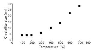
Fig. 8. Ceria crystallite size calculated for different temperatures (100-700 °C) of the final heat treatment.
