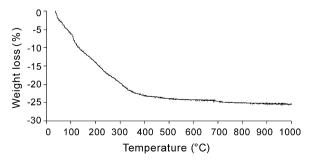
Fig. 5. Thermogravimetric analysis of the hydrated deposit just after the electrochemical impregnation (-40 A m<sup>-2</sup>, 10 min at room temperature).
