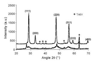
Fig. 4. XRD diagrams obtained after impregnation ( $-40 \text{ A m}^{-2}$ , 10 min at room temperature) (bottom diagram) and after final heat treatment (1 h at 700 °C) (upper diagram).
