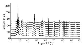
Fig. 6. XRD patterns obtained at different temperatures (100-700 °C) of the final heat treatment.
