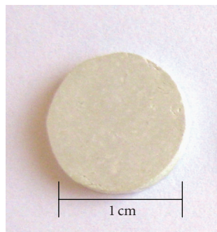
FIGURE 6: Picture of the BCZY09 CS pellet, after polishing.
