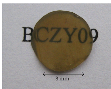
FIGURE 4: Picture of the BCZY09 SPS pellet, after polishing.
