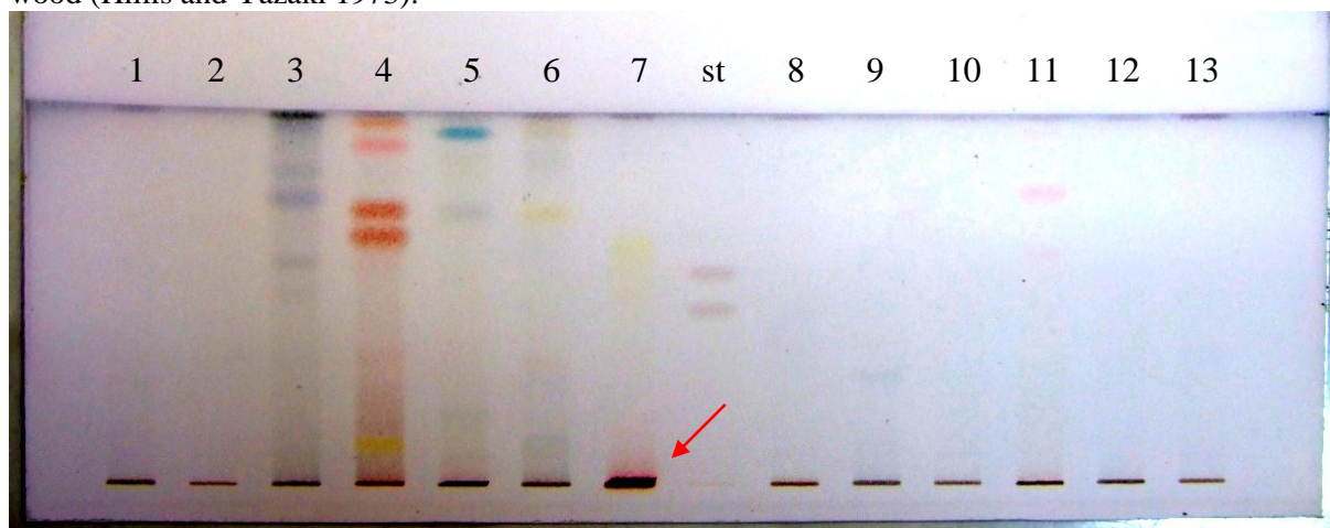
Fig. 1. Derivatization with vanillin-H 3 PO 4 . St (followed from the bottom up: (-)-epicatechin (red), (+)-catechin (red)). Samples and respective numbers: 1: Bilinga, 2: Bongossi 3: Canalete 4: Doussié 5: Makassar 6: Mansonia 7: Merbau 8: Okoumé 9: Ramin 10: White lauan 11: Wengé 12: Zebrano 13: Danta.
