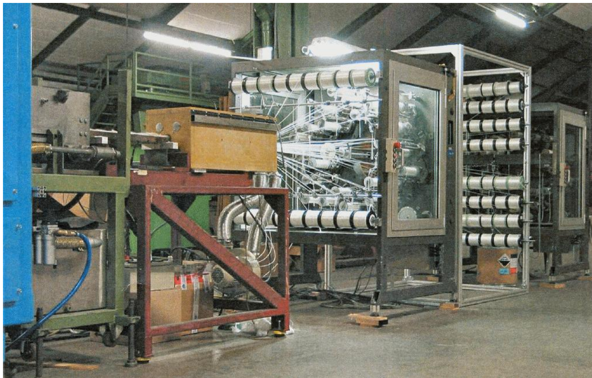
Fig. 9 Braid pultrusion setup, © Institute for Textile Technology and Process Engineering Denkendorf.
