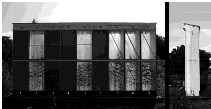
Figure 2: Experimental greenhouse with nine growth chambers (left: front view, right: side view). The chambers are about 4,5m high and have a floor space of about 0,9m x 1,2m. In each chamber there are six plants. The dividing walls are made of light tide white boards. The outer walls are made of greenhouse film (folitec UV5.)
