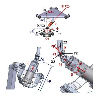
Fig. 2. Delthaptic handle design and parameterization
