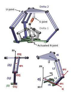
Fig. 1. Delthaptic schematic drawing and parameterization
