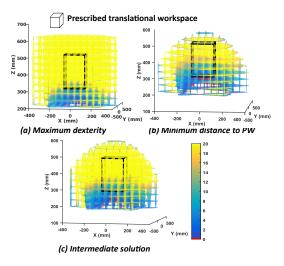
Fig. 5.  $|\det(\mathbf{J})|$ , constant orientation workspace  $[\phi, \theta, \psi] = [0, 0, 0]$
