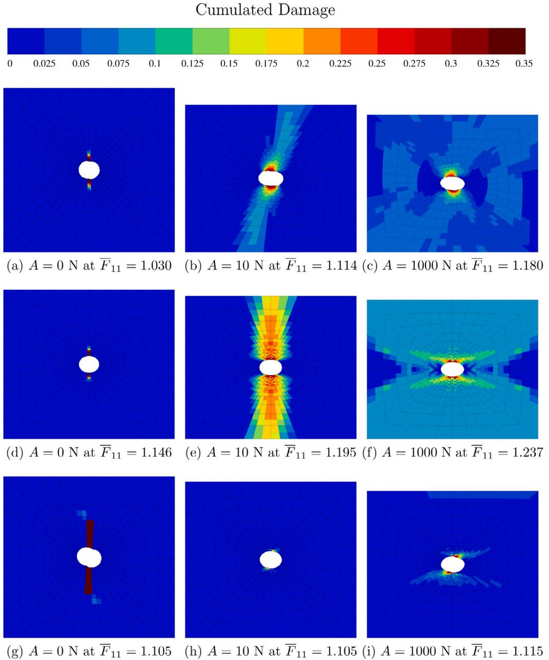
Fig. 5. Influence of parameter  $A$  on damage variable fields for crystal directions  $([100],[010],[001])$  in (a–c),  $([110],[\bar{1}10],[001])$  in (d–f) and  $([111],[\bar{2}11],[0\bar{1}1])$  in (g–i).  $A = 0$  N in (a, d, g),  $A = 10$  N in (b, e, h) and  $A = 1000$  N in (c, f, i).  $H_y$  is set to  $10^4$  MPa.
