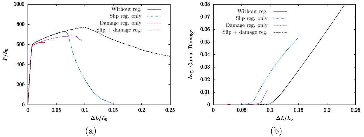
Fig. 2. Influence of the chosen variable for gradient regularization on (a) the stress–strain behavior and (b) average cumulated damage evolution for a  $[100] - [010] - [001]$  crystal orientation.  $H_x$  is set to  $10^4$  MPa.
