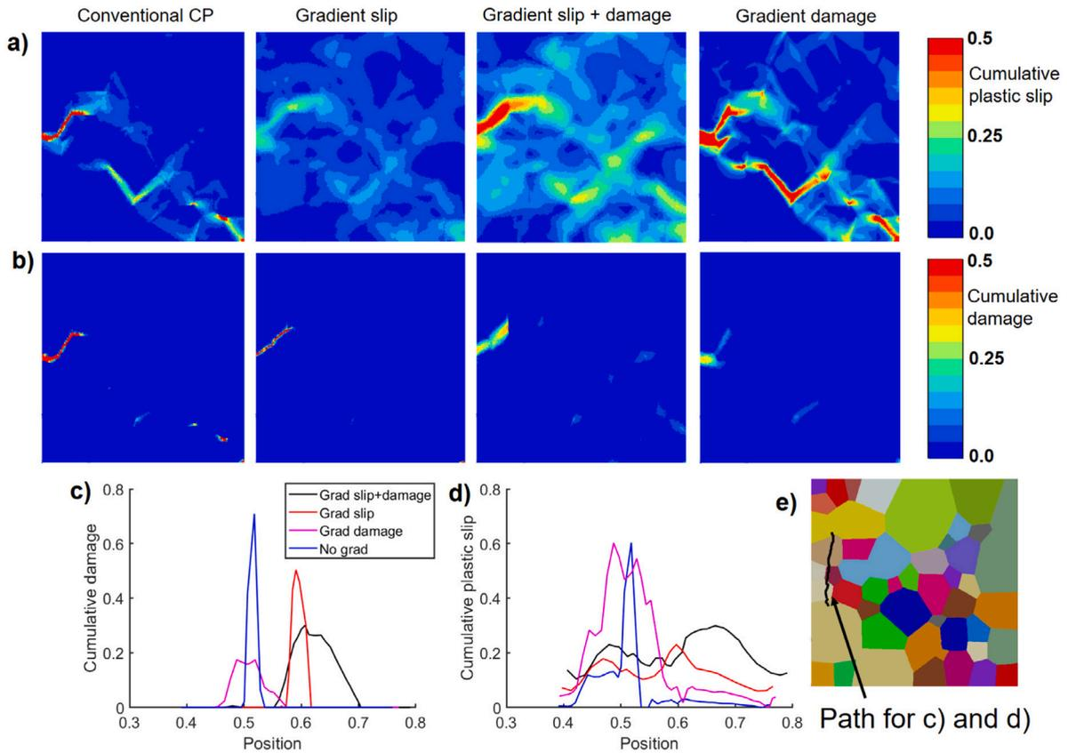
**Fig. 11.** (a) Slip localization and (b) damage strain during uniaxial tension. Plot over predefined path on damaged region (c) cumulative damage strain, (d) cumulative plastic slip distribution, and (e) prescribed path for position plots on polycrystalline mesh on (c–d). Contours are plotted on undeformed configuration for clarity.
