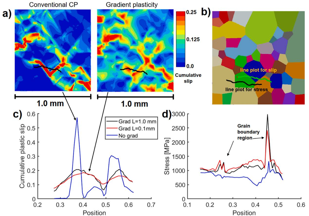
**Fig. 8.** (a) Plots over predefined path (in black) cumulative plastic slip contours for conventional and strain gradient cases, (b) slip and stress line plots on polycrystalline microstructure, (c) cumulative plastic slip profile, and (d) stress distribution over the line plots. Position coordinates of the gradient case with scaling 0.1 (100  $\mu\text{m}$ ) are upscaled 10 times to match normal 1.0 scaling (1000  $\mu\text{m}$ ) of the polycrystal aggregate in Figures (c) and (d).
