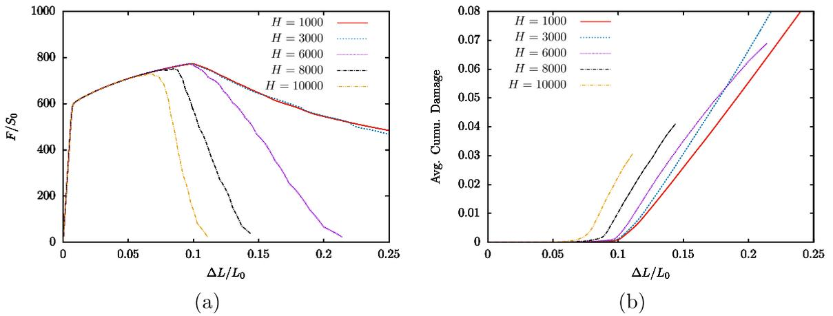
Fig. C.19. Influence of parameter  $H$  on damage onset and softening acceleration for  $[100] - [010] - [001]$  crystal orientation with  $H_x = 10^4$  MPa. Parameter  $H$  is treated as negative value to cause softening.
