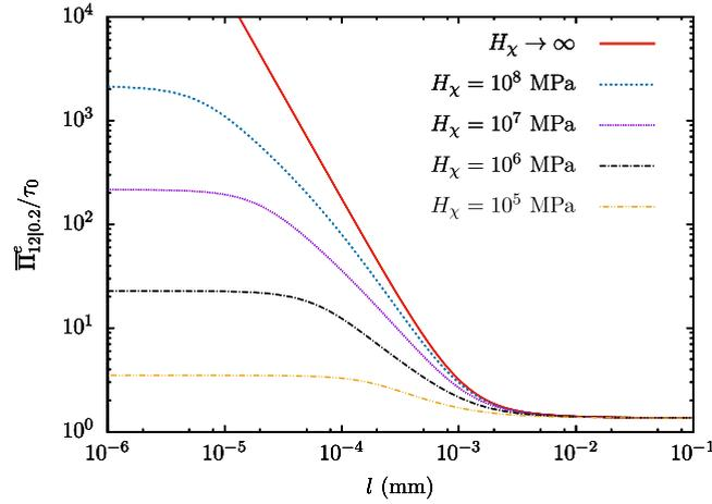
Fig. A.16. Evolution of the normalized macroscopic stress  $\bar{\Pi}_{12|0.2}^e / \tau_0$  at 0.2% macroscopic shear strain as a function of the microstructure length  $l$  for several values of the penalization parameter  $H_\chi$  with  $f_s = 0.7$  and material parameters presented in Table A.3.
