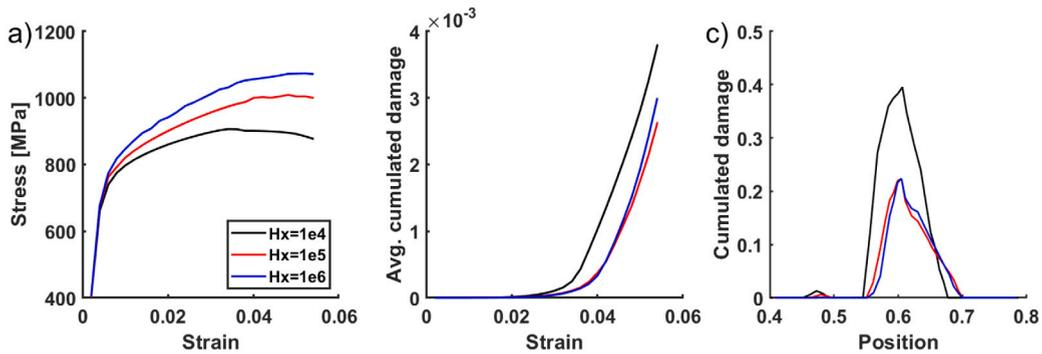
Fig. D.20. (a) Polycrystal hardening response for three  $H_x$  values, and (b) effective damage responses, and (c) line plot over a damage region at 5.5% of axial strain, using slip and damage regularization mode. Modulus  $A$  is set to  $1.0 \text{ MPa mm}^2$ .
