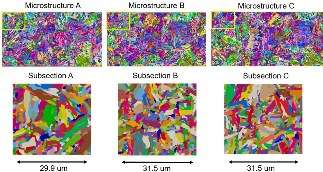
Fig. 12. Three computational microstructures sub-sectioned from different EBSD measurements.
