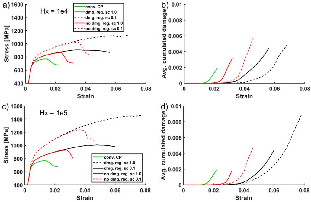
Fig. 9. (a), (c) Stress–strain evolution for two length scales with and without damage regularization, (b), (d) evolution of cumulated damage in a polycrystal, for two  $H_x$  values. Aggregate sizes 1.0 and 0.1 mm are referred with sc. 1.0 and sc. 0.1 (scale).
