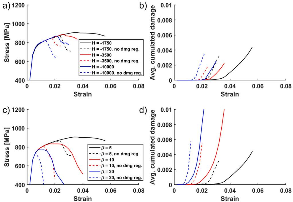
Fig. D.22. Effect of damage softening parameter  $H$  on (a) stress–strain behavior, (b) damage evolution with  $\beta = 5.0$ . Effect of plasticity–damage coupling parameter  $\beta$  on (a) stress–strain behavior and (b) damage evolution with  $H = -1750$  MPa. Micromorphic parameters are  $H_x = 10^5$  MPa and  $A = 1.0$  MPa mm<sup>2</sup>.
