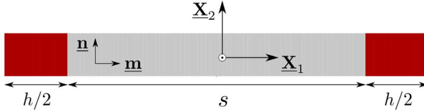
Fig. A.14. Periodic two phase laminate geometry with the soft phase (gray) of width  $s$  undergoing elasto-plastic deformations with a single slip system ( $\underline{n}, \underline{m}$ ) and the hard phase (red) of width  $h$  undergoing purely elastic deformations. (For interpretation of the references to color in this figure legend, the reader is referred to the web version of this article.)
