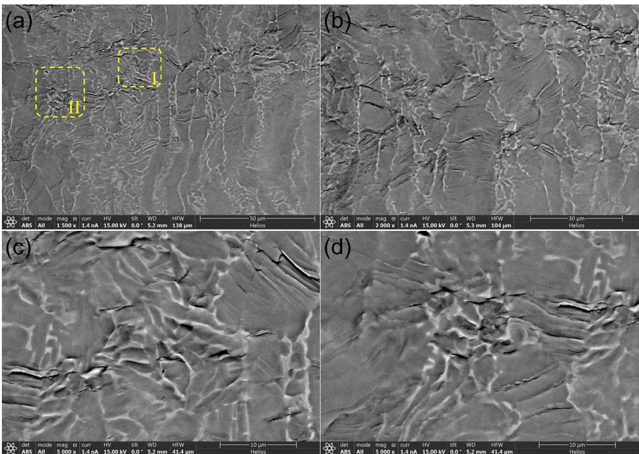
**Fig. 3.** (a) and (b) outer circumferential surface morphologies of a specimen failed due to interior crack initiation ( $\sigma_a = 580$  MPa,  $N_f = 7.43 \times 10^7$  cycles), (c) and (d) microvoids nucleated in  $\beta_t$  (magnified image of Regions I and II in (a), respectively).
