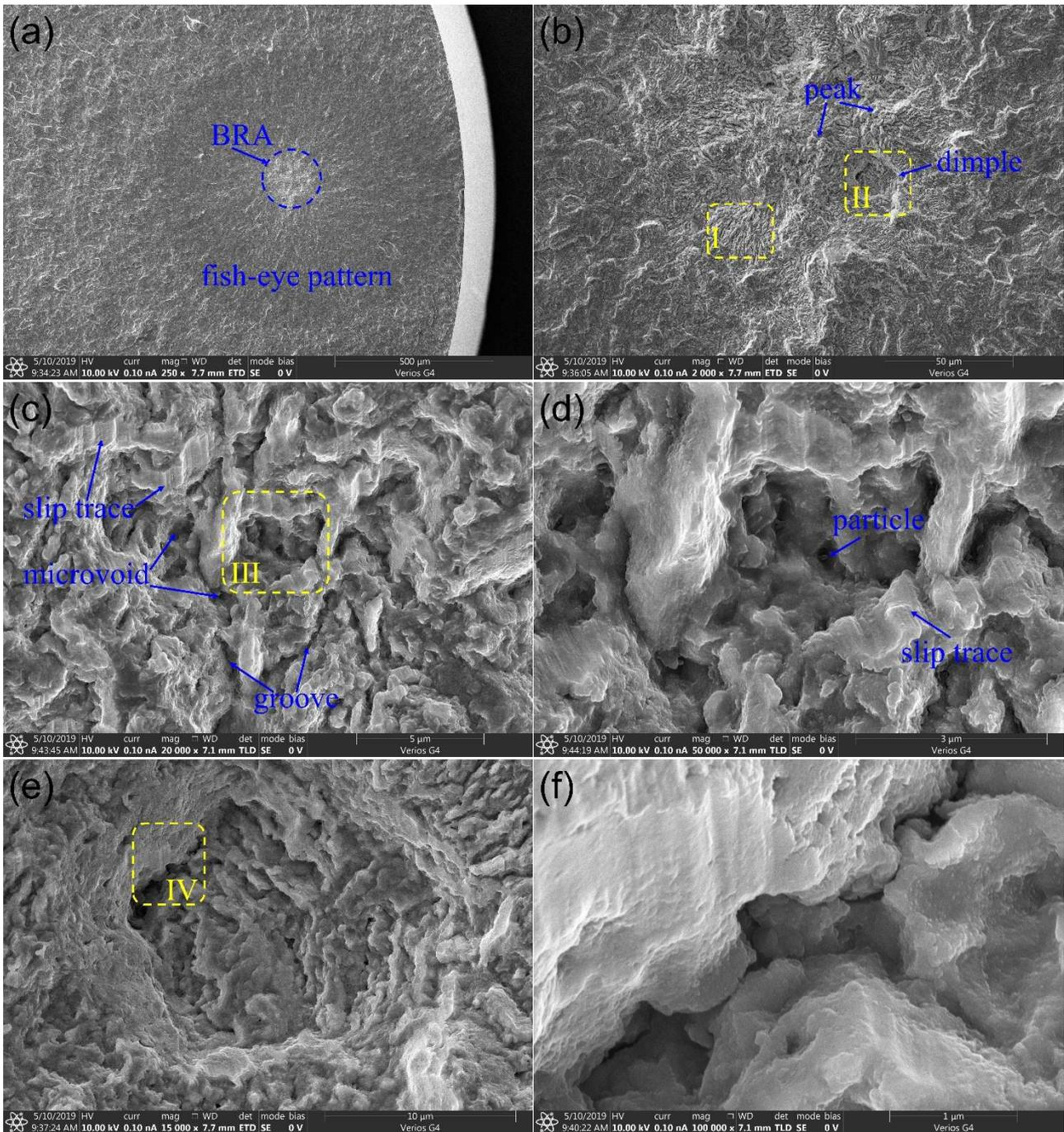
**Fig. 2.** Example of an interior-induced fracture surface ( $\sigma_a = 580$  MPa,  $N_f = 1.25 \times 10^8$ ): (a) overall view of fish-eye pattern; (b) magnified image of the bright rough area (BRA) at the center of the fish-eye pattern; (c) magnified view of Area I in (b); (d) magnified view of microvoids in Area III in (c); (e) magnified view of a dimple in Area II in (b); (f) magnified view of grooves at the dimple bottom IV in (e).
