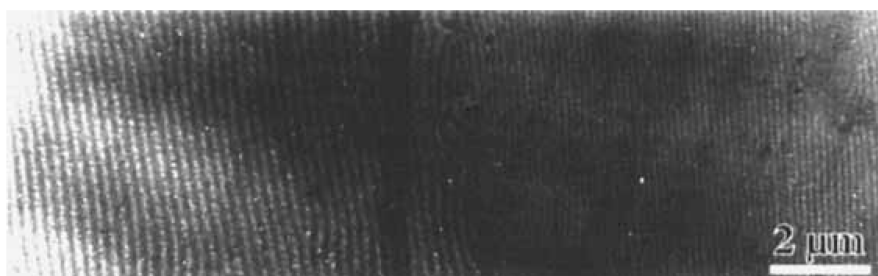
FIGURE 3 TEM micrograph of a cross-section of a sandwich-cell after 5 min of annealing
